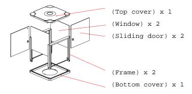
The windshield consists of 8 components as illustrated in the above drawing. If any items are missing, please contact your local distributor for assistance.
